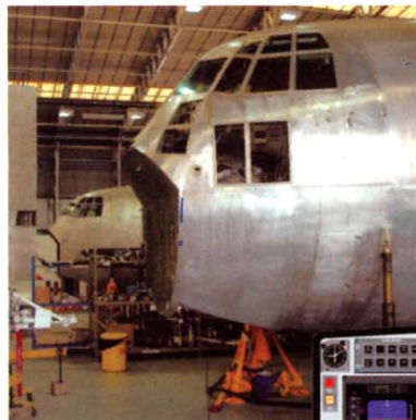
Two ex-U.S. Navy EC-130Q Tacamo aircraft (above) are being upgraded for the Netherlands, which includes the common core cockpit (right).
