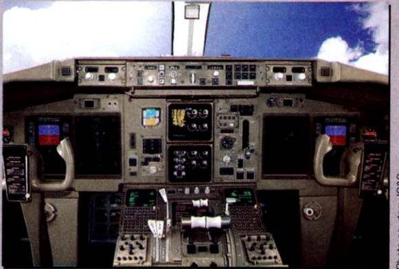
Innovative Solutions & Support Integrated Primary Flight and Navigation Display in ABX Boeing 767.
