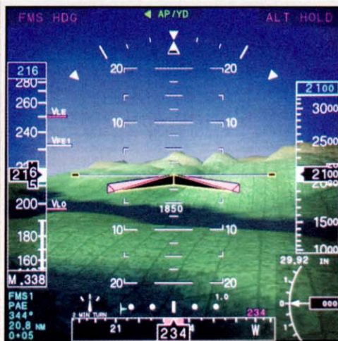
Universal Avionics' Vision 1 Synthetic Vision System offers an egocentric, or pilot's, view (shown) as well as an exocentric wingman's view.
