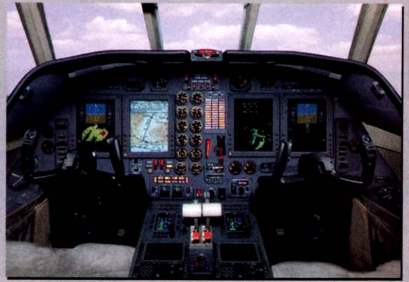
Rockwell Collins' Pro Line 21 integrated display system installed in a Dassault Falcon 200.
