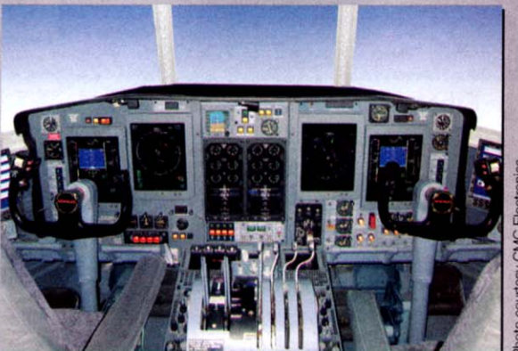
Part of C-130 cockpit retrofit for the Dubai Air Wing includes CMC Electronics' fully integrated, CMA-900 multisensor Flight Management System.
