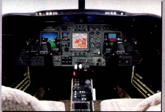
Universal Avionics flat-panel displays can be seen in Stevens Aviation's Lear 25 instrument retrofit.
