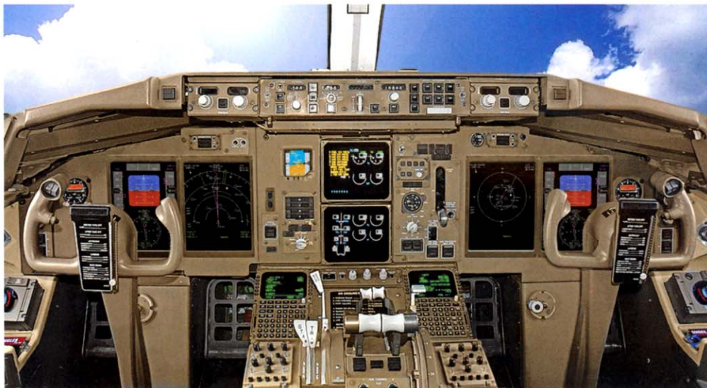
The Innovative Solutions and Support primary flight/navigation display for operators of Boeing 757 and 767 aircraft features a pilot and co-pilot suite, each containing two 6 x 8-in integrated flat-panel displays.
